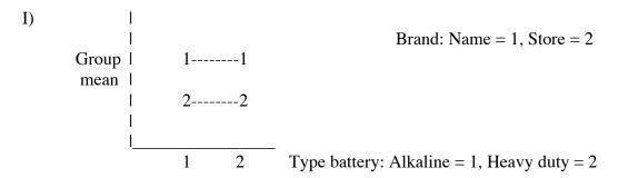
In the plot, the categorical variable "Type battery" (one of the treatment factors) is on the horizontal axis, the means of the quantitative response variable LPUC are on the vertical axis, and the points in the plot are marked by the level of the second treatment factor, "Brand." We could also form an interaction plot by interchanging the roles of the two factors – that is, put "Brand" on the horizontal axis, and mark by "Type battery."
